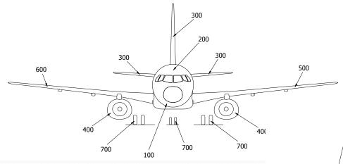
MAJOR ZONE 500 – LEFT WING MAJOR ZONE 600 – RIGHT WING MAJOR ZONE 700 – LANDING GEAR AND LANDING GEAR DOORS MAJOR ZONE 800 – PASSENGER AND CARGO COMPARTMENT DOORS MAJOR ZONE 100 – LOWER HALF OF FUSELAGE (UP TO BACK PRESSURE BULKHEAD) MAJOR ZONE 200 – UPPER HALF OF FUSELAGE (UP TO BACK PRESSURE BULKHEAD) MAJOR ZONE 300 – EMPENNAGE MAJOR ZONE 400 – POWER PLANTS AND NACELLE STRUTS
